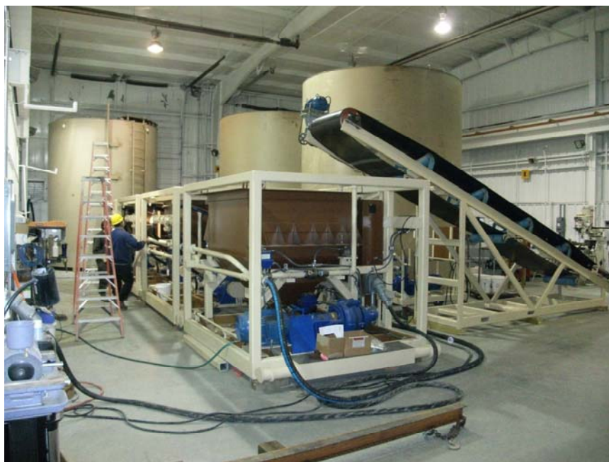
The 5tph Unit during tests in Casper, Wyoming, USA. The slurry mix tank, being fed by a conveyor, is in the foreground. Three interconnected ablation modules are positioned immediately behind the mix tank. Three water storage tanks are evident in the background.
